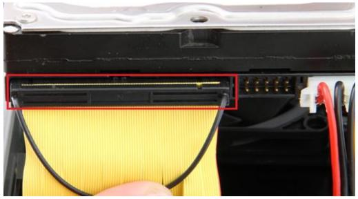
Insert the hard into the enclosure, as shown below:
